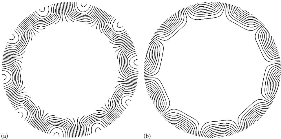
Fig. 4. Smoothed isolines of the derivatives of the deflection (a—in the radial direction; b—in the angular direction).
