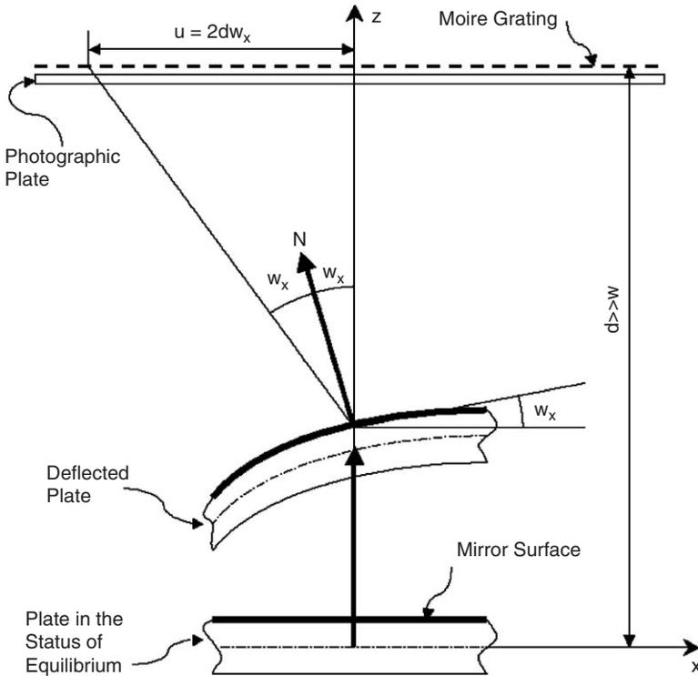
Fig. 1. Schematic diagram of reflection moiré measurement set-up.
