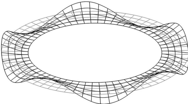
Fig. 2. The tenth eigenmode of the centrally clamped disk.
