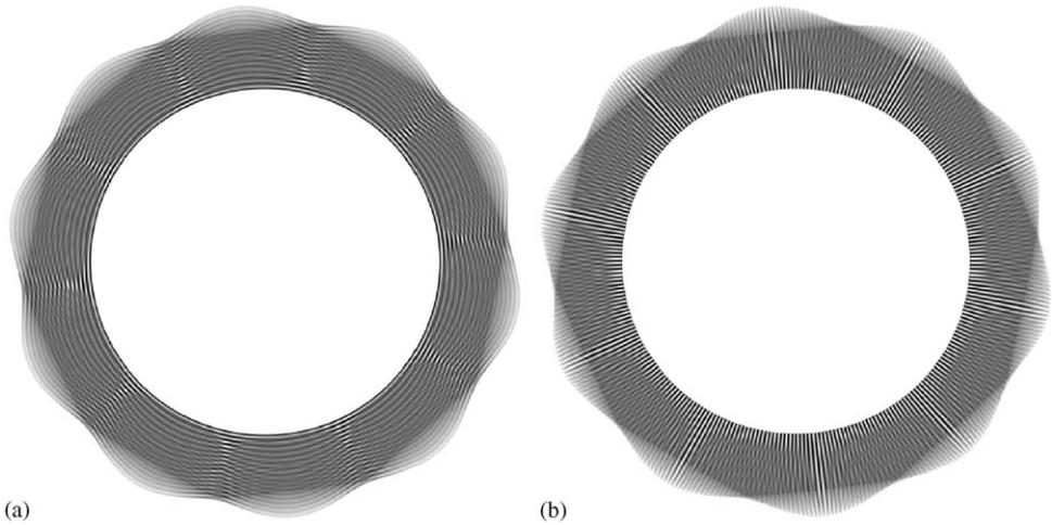
Fig. 5. Time average reflection moiré images (a–radial grating; b–angular grating).
