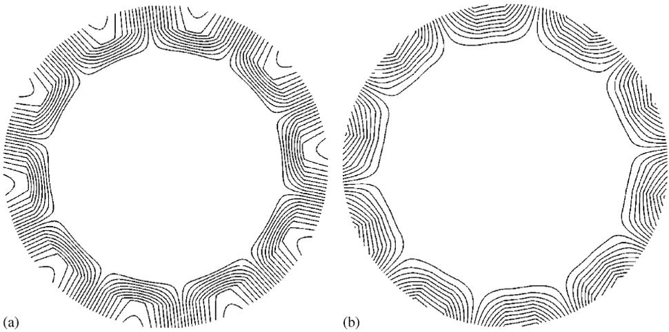
Fig. 3. Unsmoothed isolines of the derivatives of the deflection (a—in the radial direction; b—in the angular direction).
