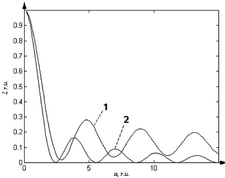
Fig. 2. The decay of intensity of illumination at increasing amplitude  $a$  (horizontal axis— $a$ ; vertical axis—intensity of illumination): (1) for oscillations described by Eq. (3) at  $c = 0.5$ ; (2) for harmonic oscillations.
