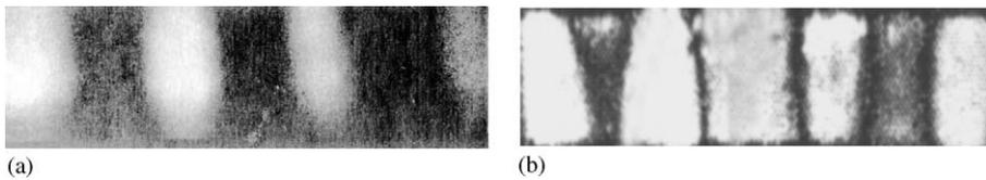
Fig. 8. Time average holograms of cantilever beams: (a) representing cantilever without limiter (no drain contact); (b) cantilever with limiter (drain contact representing  $c = 0.5$ ).
