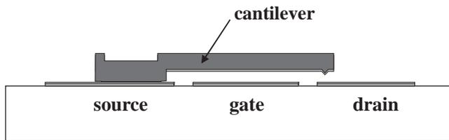
Fig. 6. Schematic presentation of the switch construction.
