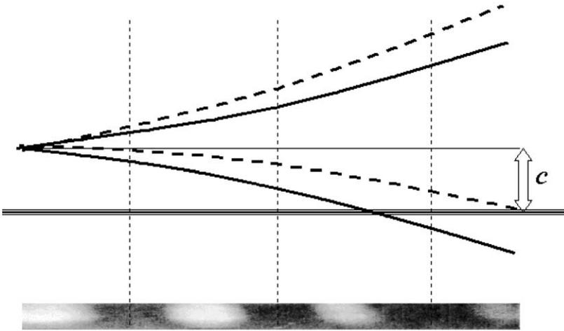
Fig. 9. The procedure of reconstruction of the cantilever motion: (solid lines) correspond to the assumption that the vibrations are harmonic; (dashed lines) the assumption that the clearance between the tip and the drain is  $c$ .
