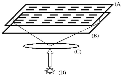
Fig. 7. The schematic diagram of the holographic set-up for recording Denisiuk hologram: (A) the array of cantilevers; (B) holographic plate; (C) lens; (D) laser light source.
