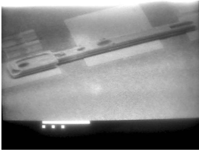
Fig. 5. SEM microphotograph of the microelectromechanical switch. Mark size 100  $\mu\text{m}$ .
