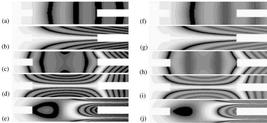
Fig. 4. Numerically reconstructed interference fringes for the first five eigenshapes; a, b, c, d, e—representing harmonic vibrations of cantilever without limiter (no drain contact).
