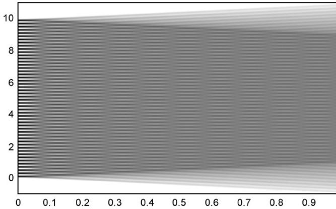
Fig. 1. A pattern of time-averaged fringes produced by the harmonic moiré grating.
