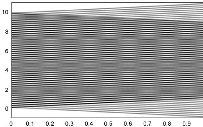
Fig. 2. A pattern of double exposure fringes produced by the harmonic moiré grating.
