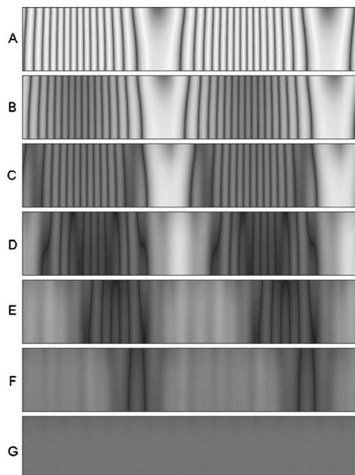
**Fig. 6** The smoothed digital time-averaged holographic image of the traveling wave: exposure time (a) 1/64 period; (b) 1/32 period; (c) 1/16 period; (d) 1/8 period; (e) 1/4 period; (f) 3/4 period; (g) 1 period.
