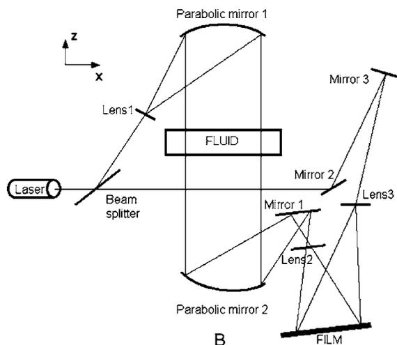
**Fig. 1** Schematic diagram of the experimental setup: (a) geometry of the fluid bath; (b) optical setup.
