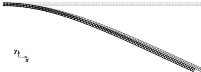
Figure 3. Maximum deflections from the state of equilibrium: light grey mesh—state of equilibrium; grey mesh—linear system; black mesh—nonlinear system.
