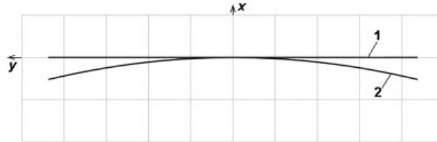
Figure 4. Trajectories of oscillation of the driven node: 1—linear system; 2—nonlinear system.
